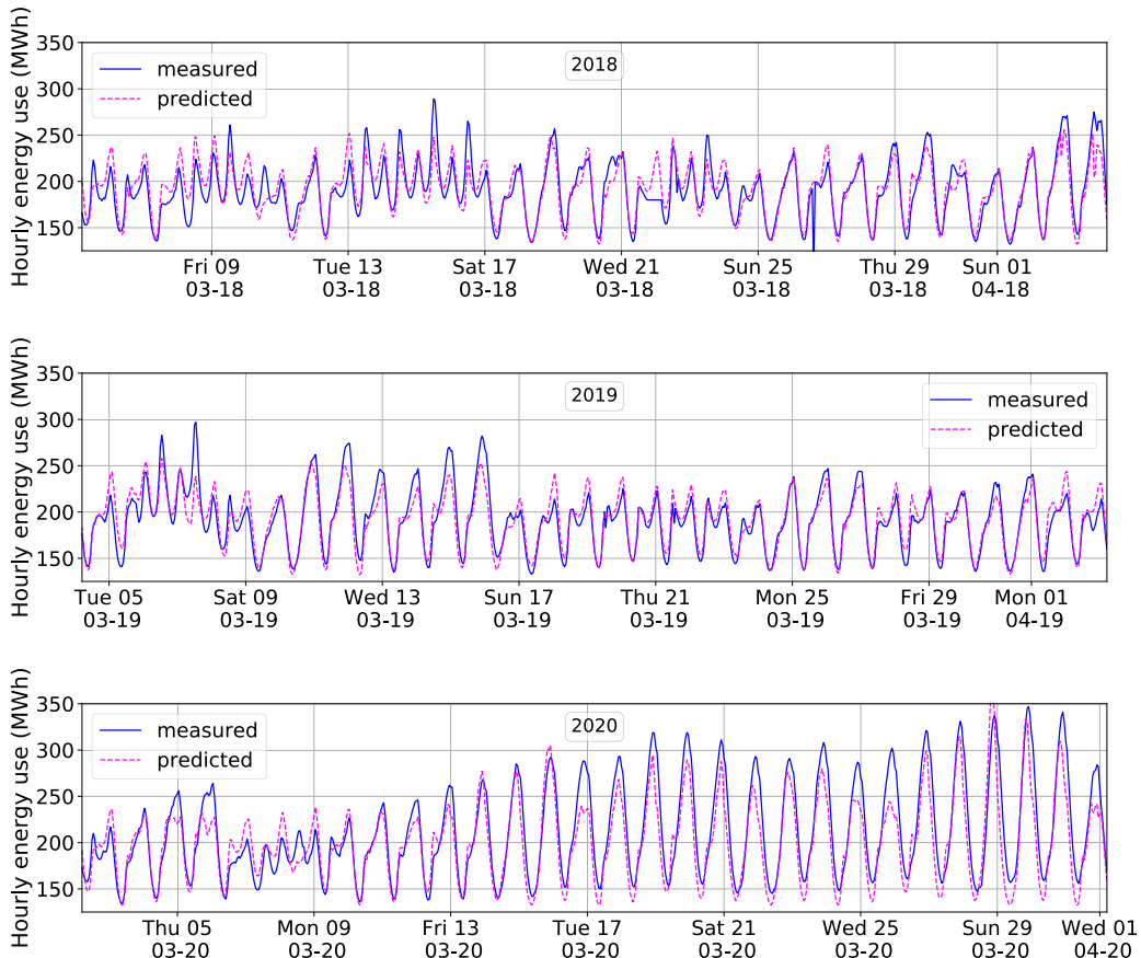
FIGURE 12. Hourly demand prediction for 3 distinct years by the model (1) trained with 2019 March data. The x-axis starts on the first Monday of March for each year.
