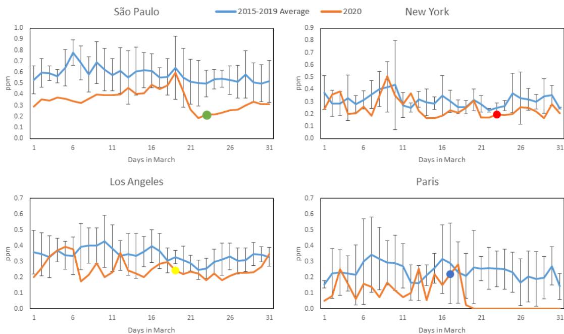
Figure 2. CO concentration profiles during March 2020 (Orange) compared to average and standard deviation of March concentrations over the previous 5 years (Blue) for the four studied cities (most significant COVID-19 intervention date indicated with colored dot). All available station data used for each city (see Section 2.2).
