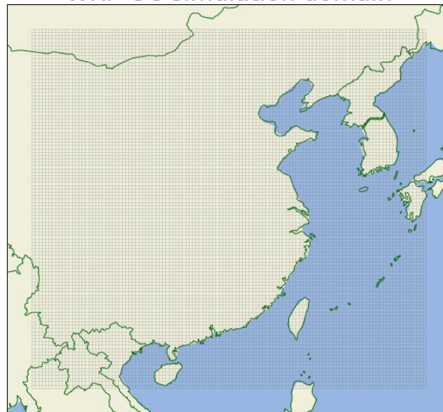
Figure A1. Domain setting of WRF-GC. Gray bordered grids represent the model grids of 27 \times 27 \text{ km}^2 resolution.
